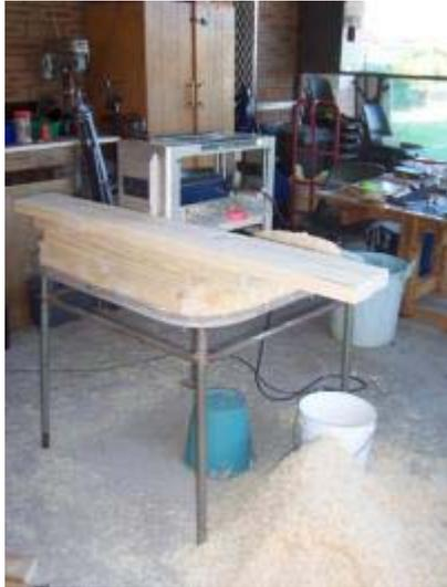
The stock was then jointed and passed through the thicknesser until the dimensions were 80mm X 40mm and the planks were 20mm X 145mm, square and flat.
