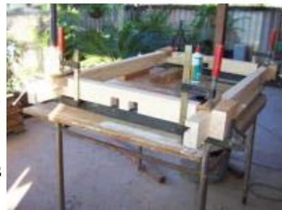
the centre doesn't end up shorter than the ends. At this stage cut matching biscuit slots in the joining edge of the two ends and the centre inserts. Cut two slots to each flap of the centre for a total of four and glue biscuits into one end and the opposite edge of the centre. These are the locating slots for mating the table sections. Dowel or brass pins could be used instead.
