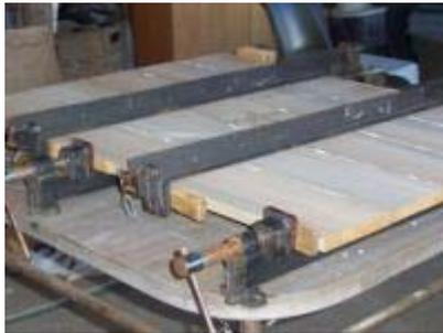
Because the table was made from packing timber the wood was back sawn which lends to wood cupping, for this reason I tried to join the wood with the grain rings in alternate
