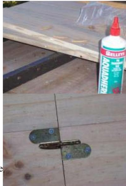
The centre is cut in half and 6mm slots are cut using the router in both halves 120mm from either edge for
