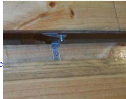
The position of the pivot hinge folded down (above) half way up (left) and fully opened (right). Note the biscuit slots in the extension to align it with the ends.
